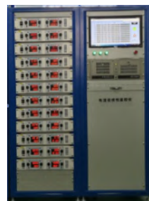
PID Test Power Supply
